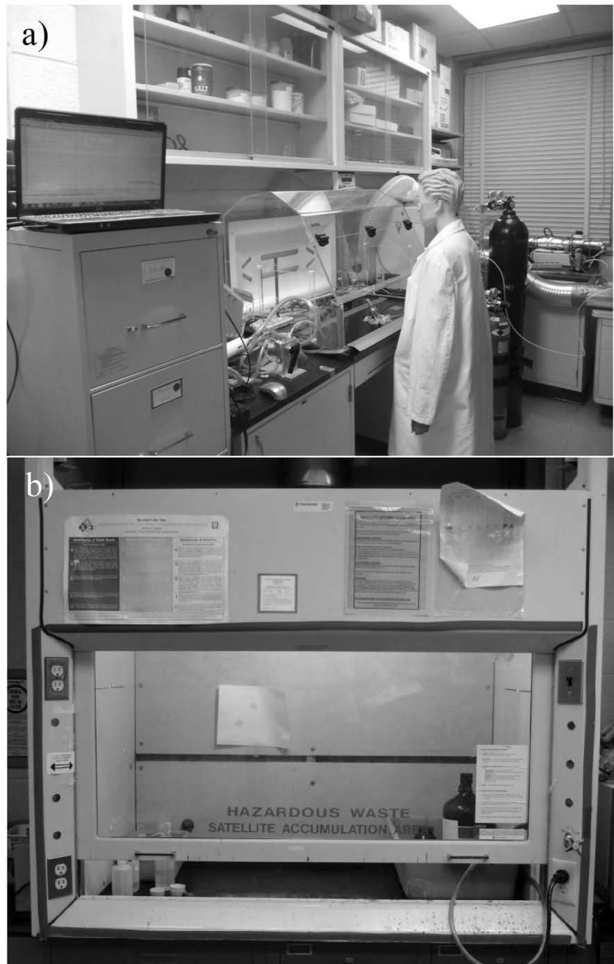
Fig. 1 Mannequin and hood setup for experiments. a) Nano hood. b) CAV hood
