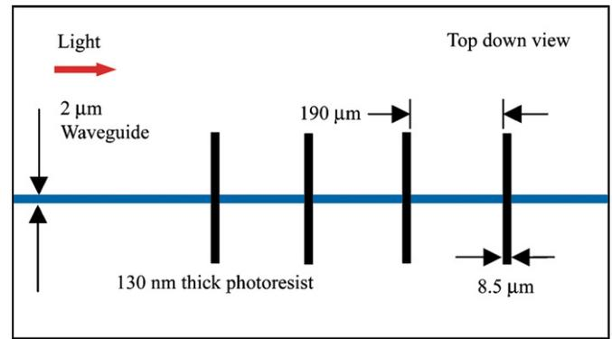
Fig. 2. Mask geometry for fabrication of uniform photoresist features patterned on the waveguide.
