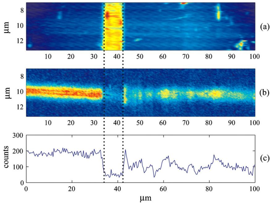
**Fig. 4.** Experimental light response to the second photoresist features in a series of four. Light propagates from left to right. (a) Topography of 2.0 μm wide waveguide with 14 nm etch depth. Feature size is ≈8.5 μm in length and 130 nm thick, (b) surface light intensity measured with NSOM, and (c) total light measured in photon counts carried in the waveguide after subtracting the background.  $\Delta P = 76.9\%$ . Dashed lines indicate location of patterned feature.
