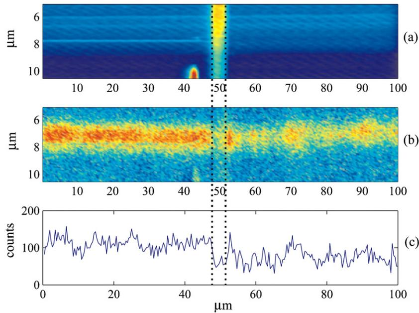
**Fig. 7.** Light response to small photoresist feature. Light propagates from left to right. (a) Topography of 2.0  $\mu\text{m}$  wide waveguide with 14 nm etch depth. Feature size is  $\approx 3.9 \mu\text{m}$  in length and 70 nm thick, (b) surface light intensity measured with NSOM, and (c) total light measured in photon counts carried in the waveguide after subtracting the background.  $\Delta P = 45.6\%$ .
