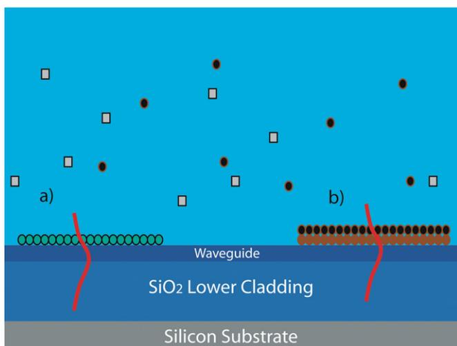
**Fig. 1.** (a) Evanescent field profile for probe region with no bound analyte. (b) When probes capture analyte from solution, the evanescent field profile shifts up out of the lower cladding.
