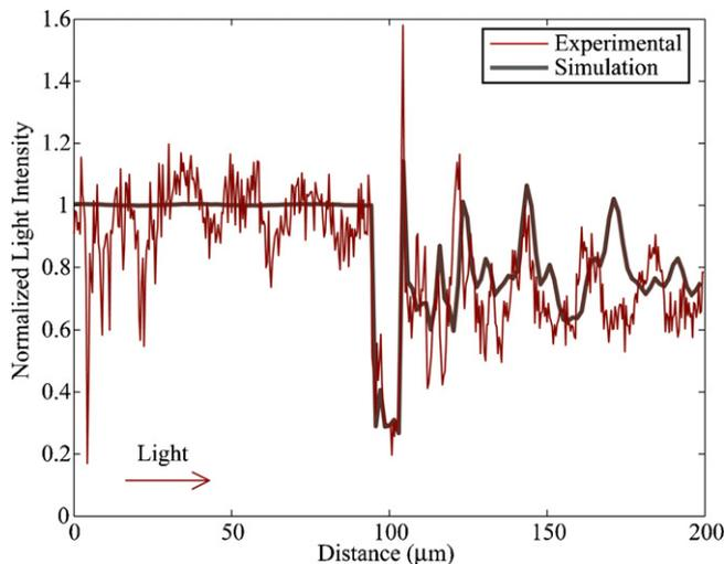
**Fig. 5.** An overlay of experimental response and simulated response to the 130 nm thick, 8.5 μm long photoresist feature. Light sampled along the top surface of the core and photoresist feature.  $\Delta P = 51.9\%$ . Light propagates from left to right.
