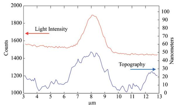
Fig. 3. Cross-section plot of the light intensity (top) and topography (bottom) of an approximately  $3\ \mu\text{m}$  wide ridge waveguide etched 14 nm. Light profile indicates a single bound mode.
