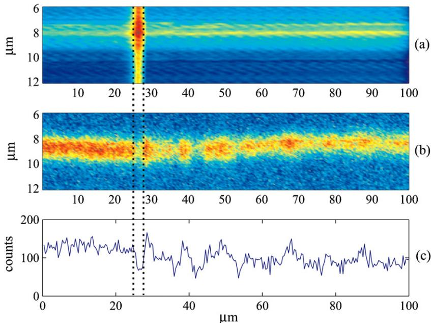
**Fig. 8.** Light response to the smallest fabricated feature. Light propagates from left to right. (a) Topography of 2.0  $\mu\text{m}$  wide waveguide with 14 nm etch depth. Feature size is  $\approx 2.7 \mu\text{m}$  in length and 50 nm thick, (b) surface light intensity measured with NSOM, and (c) total light measured in photon counts carried in the waveguide after subtracting the background.  $\Delta P = 26.4\%$ .
