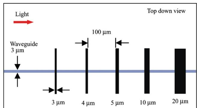
**Fig. 6.** Mask geometry for fabrication of variable size photoresist features patterned on the waveguide.
